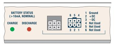
Figure 6 Front panel detail showing output connector and pinout chart
