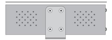
$\textbf{Figure 2} \quad \text{Right side view of Model 730 with wall-mount bracket attached}$
