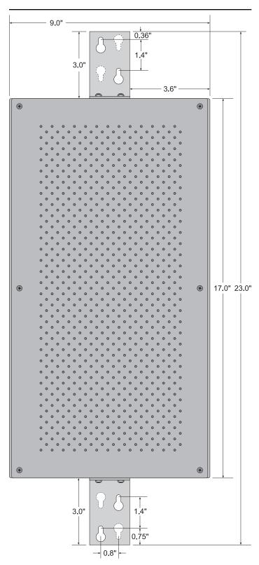
Figure 3 Recommended Model 730 wall-mount configuration
