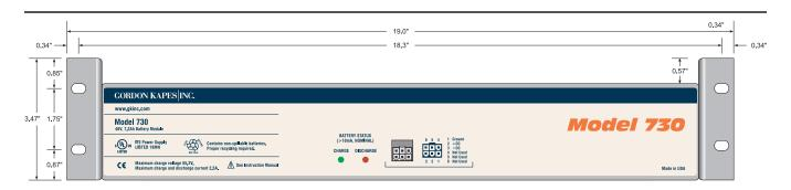
Figure 5 Front view of Model 730 with 19-inch rack-mount brackets attached
