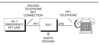
Figure 2 Installation with SL-1 Emergency PFT.
